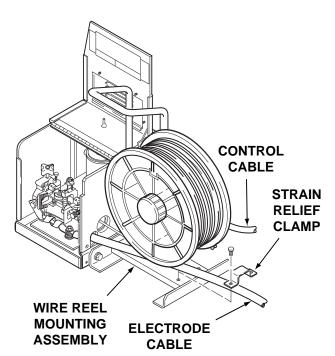
FIGURE A.3 – LN-742 WIRE FEEDER TO LINCOLN POWER SOURCE – CONNECTION DIAGRAM.
